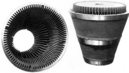
cast steel paper mill stockbreaker
