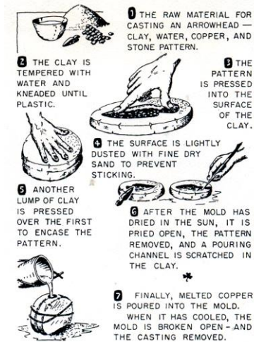
FIGURE 2.2 Steps in casting an arrowhead (used by the primitive people).
